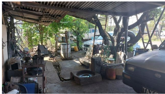
Figure 5 (below). View to the right side of Jimi's workshop where much of the sinking of the Pans take place. The far mid-centre shows a white drum in the process of being sunk with a hydraulic hammer. These open spaces provide a wonderful ambience and tranquil atmosphere for working and teaching. (Photo taken by Louise C.F. Shah)
