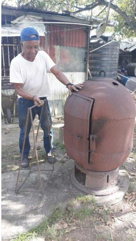
Figure 4 (left). Jimi's shrewd use of a recovered buoy from the sea and re-purposed as an 'oven' to heat Pans ahead of tuning. When the Pan has been heated sufficiently (~8 -10 minutes), the ramp (in his right hand) is laid at the door of the buoy and a metal rod used to drag the heated drum out of the oven and on to the ground where cold water is immediately poured on it to temper the metal. (Photo taken by Louise C.F. Shah)
