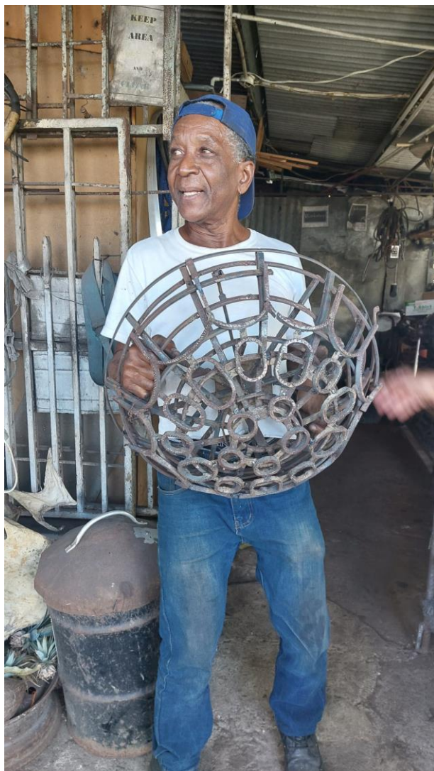
Figure 3. Jimi proudly displays his 'Stamper' for grooving the pan that is under development. The complexity and immense intricate work serve to also highlight Jimi's craftsmanship and in particular his dexterity with the process of welding. (Photo taken by Louise C.F. Shah)
